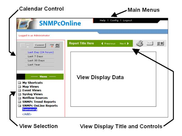
SNMPc data such as map topology, map drawings, event log entries, and trend statistics are shown in the *View Display Data* frame. This frame can display a variety of data formats including tables, graphs and custom dashboards. The remaining frames contain control tools that maintain a consistent format at all times. Settings in the control tools determine what is displayed in the *View Display Data* frame.
