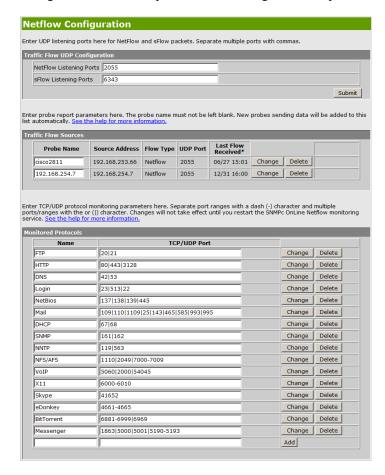
Enter a list of comma separated UDP ports that SNMPc should listen for Netflow and SFlow data in the first two edit boxes. The defaults are 2055 and 6343, respectively.
