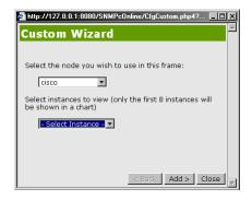
For graph displays you can have up to eight instances per cell. Use the *Instances* link to add more instances. Each node/instance pair is listed in the cell configuration screen. Use the *Delete Graphic* to the left of the node/instance name to remove an instance from the cell.
