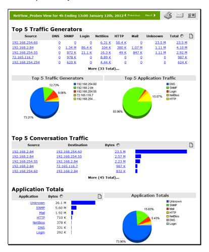
Use the *More (nn Total)*... link below a table to expand the table to all contents. In the case of the *Application Totals* table this expanded view also shows unknown applications by TCP/UDP number.
