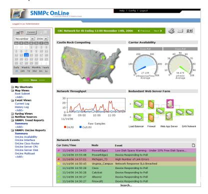
Visio drawings are created or imported using the included *MapDraw* tool. Each drawing is associated with an SNMPc OnLine *Map View*. You can also create customized dashboard views that include a Visio map drawing along with other SNMPc OnLine elements such as graphs, bar charts, data tables and event log views.
