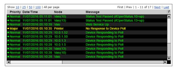
When viewing acknowledged (History) events, note that the view only shows events within the selected calendar control time period. This is different than how SNMPc typically shows events. When viewing Current events the selected time period is ignored. The number of events shown in the scroll controls at upper right of the view represents the entire number of active events.
