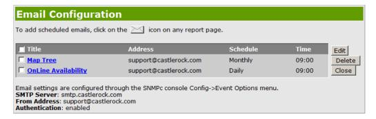
You can access this page at any time from the *Email* selection of the *Config* menu at the top right of the SNMPc OnLine main window. Select one or more entries and press the Edit button to change schedule settings or press the Delete button to remove the entry.
