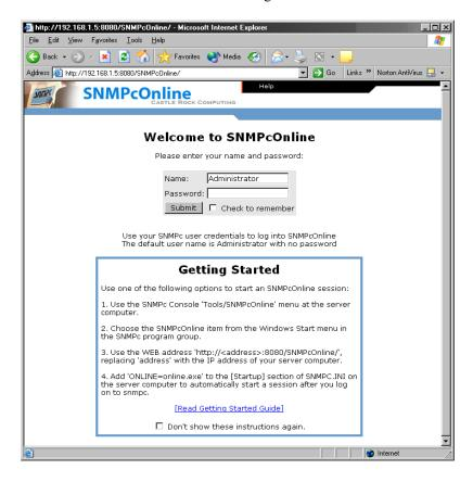
To log in, enter an SNMPc username and password. If you are using a new install of SNMPc the default username is *Administrator* with no password (i.e., blank).
