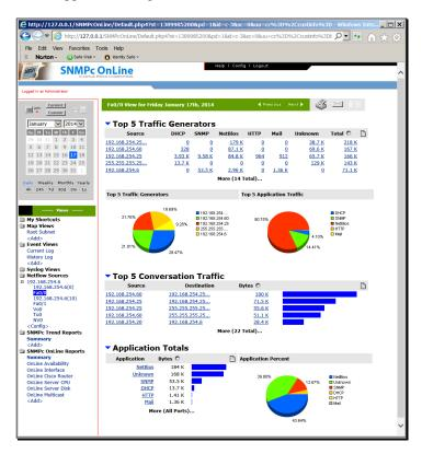
Utilizing NetFlow and sFlow enabled switches and routers in the network from manufacturers including Cisco, HP, Juniper and Allied Telesyn. SNMPc OnLine delivers network wide traffic insight without requiring the overhead of deploying separate hardware probes.
